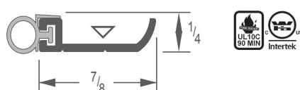
Jamb-type weatherstrip, with black vinyl bulb seal. Slotted holes for ease in adjustment.
