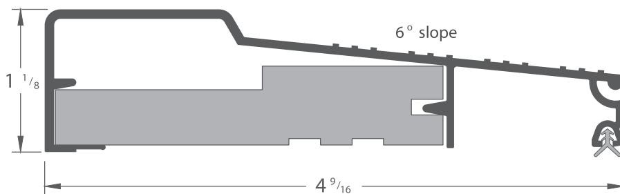
Full length wood or composite insert for glue down or nail-on applications
