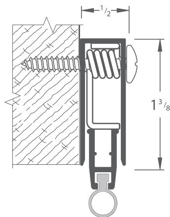
**Surface mount automatic** door bottom, pliable seal, 1/2" max. drop.
