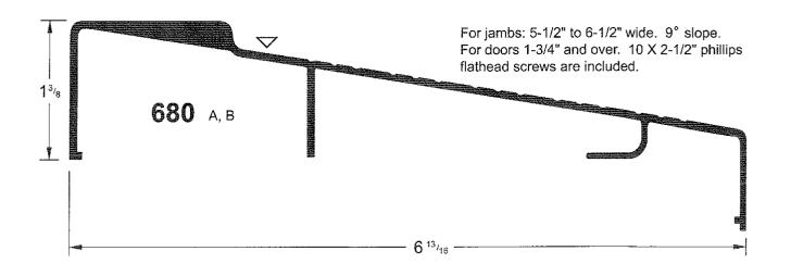
COMBO ALUMINUM PRODUCTS, EL CAJON, CA Tel (619) 447-9200 (800) 457-7500 Fax (619) 442-4558 ✓ Indicates location of standard fastener hole.
