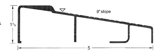
COMBO ALUMINUM PRODUCTS, EL CAJON, CA Tel (619) 447-9200 (800) 457-7500 Fax (619) 442-4558 ▼ Indicates location of standard fastener hole.
