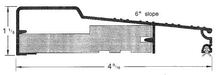
Full length wood or composite insert for glue down or nail-on applications
