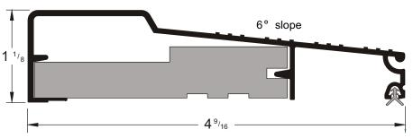
Full length wood or composite insert for glue down or nail-on applications
